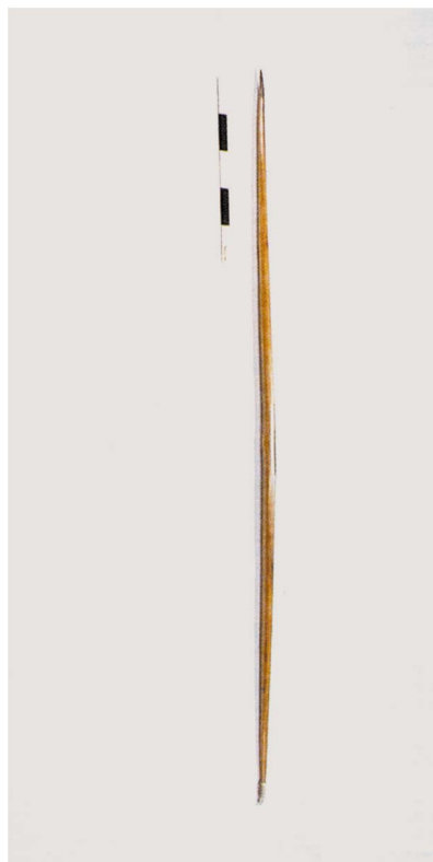
Plate 1 Occasionally waterlogged wood can be air dried without the use of consolidants, as is the case with this long bow from the Tudor warship Mary Rose , which sank in 1545 (© The Mary Rose Trust, by permission)
