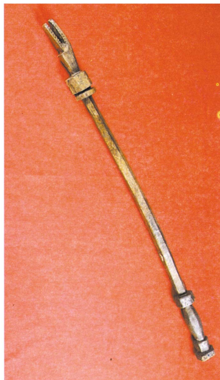
Plate 2 This linstock from the Mary Rose demonstrates the most commonly used conservation technique for small artefacts, namely freeze drying after impregnation with PEG (© The Mary Rose Trust, by permission)
