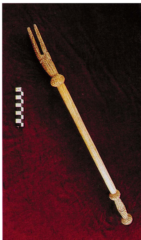
Plate 3 A technique finding increasing favour amongst conservators is impregnation with sugars. This can give a light, natural appearance to conserved wood, without the greasy texture sometimes evident on artefacts conserved using PEG. This is demonstrated here by the use of mannitol on another linstock from the Mary Rose (© The Mary Rose Trust, by permission)
