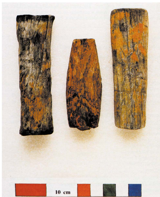
Plate 4 Treatments using PEG and sugars are unsuitable for wood/iron composite artefacts. These knife handles are from the Elizabethan warship Makeshift , which sank in 1592, and have been conserved by the author, using the supercritical drying technique. The remains of the iron blade can be seen projecting from the handle in the centre.
